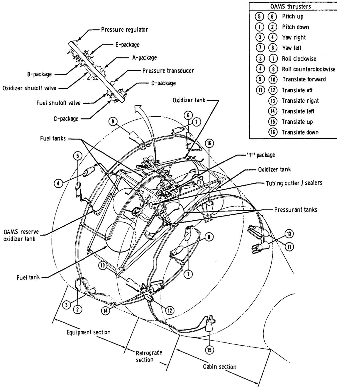
Figure 3.1-3. - Orbital Attitude and Maneuver System.
