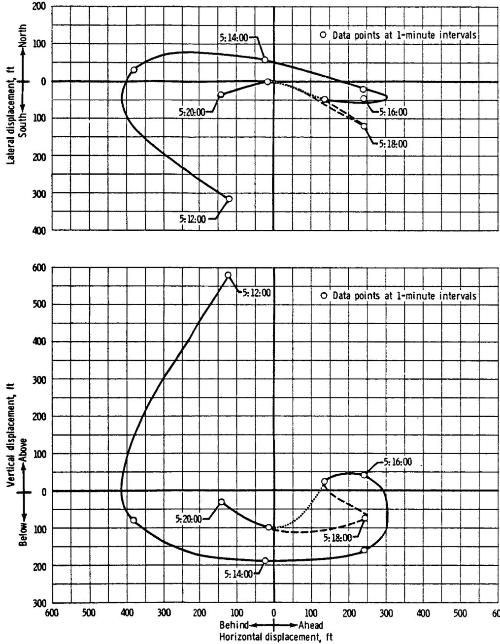
Figure 5.1.5-16. - First rendezvous final approach (expanded scale).
