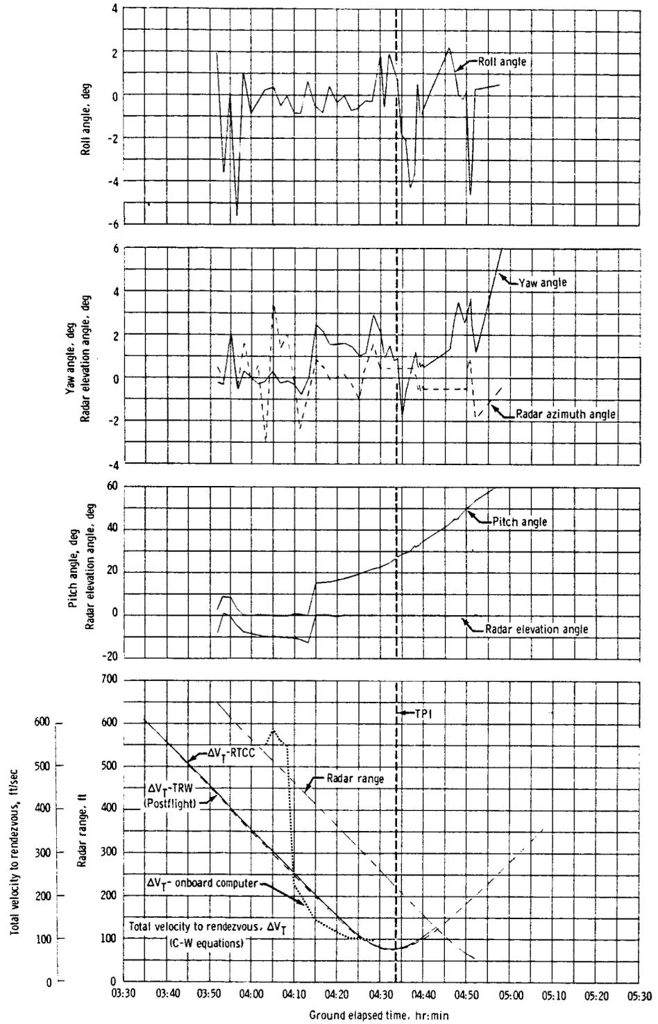
Figure 5.1.5-8. - Computer data for the closed-loop rendezvous.
