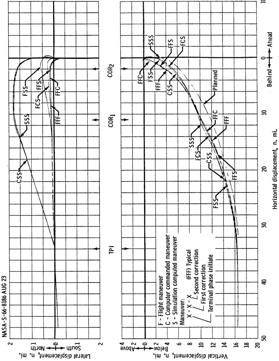
Figure 5.1.5-14. - First rendezvous simulations, with fixed platform misalignment.
