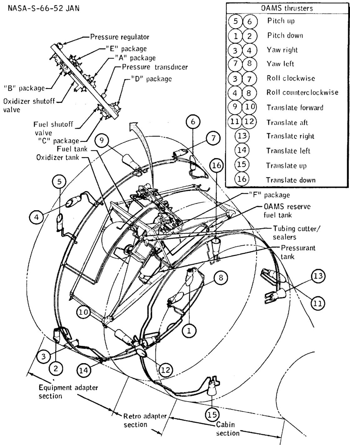
Figure 3.1-10. - Orbital attitude and maneuver system.
