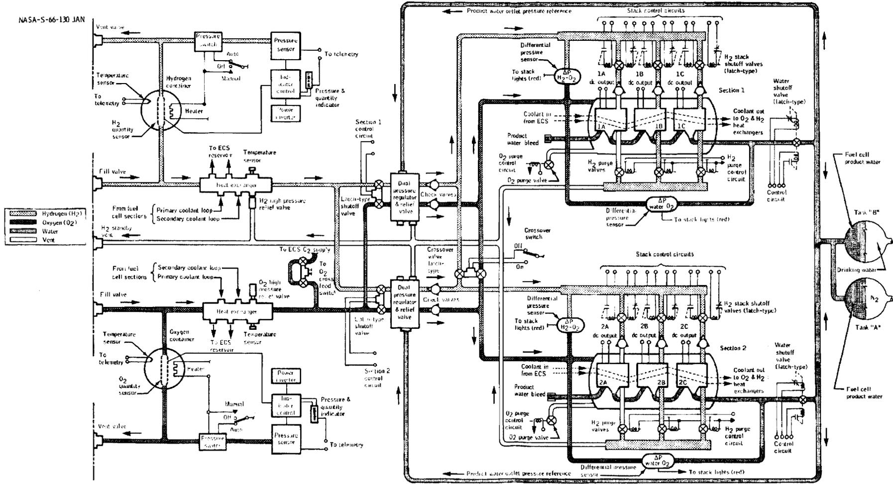
Figure 5.1-3. - RSS/fuel cell system functional diagram.
