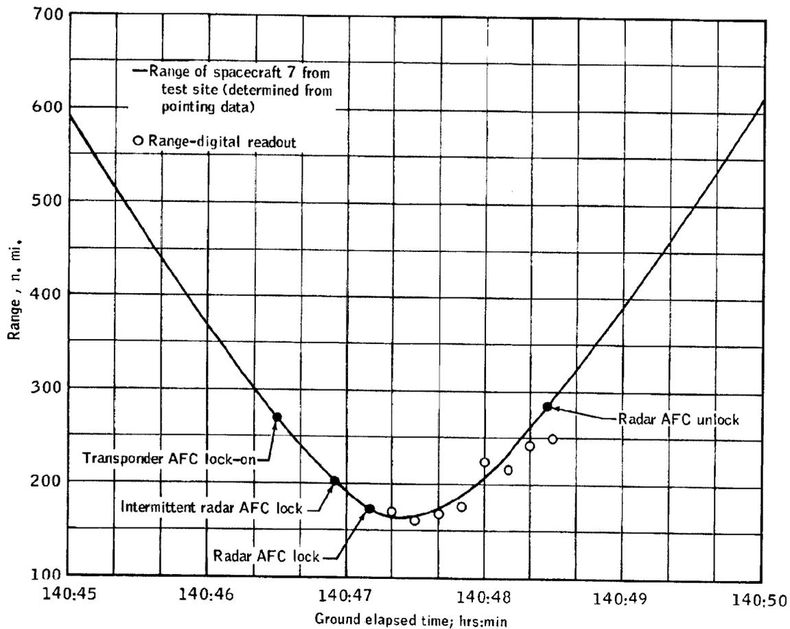
Figure 5.1.5-4. - Transponder tracking test results.
