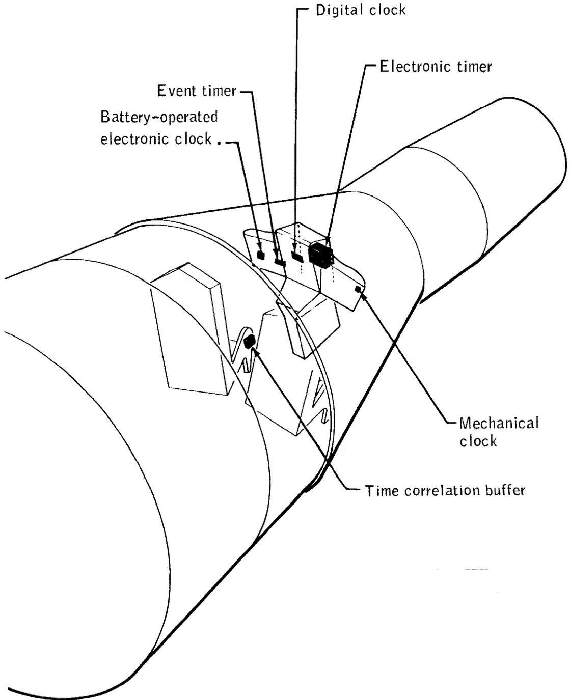
Figure 3.1-6. - Time reference system equipment locations.
