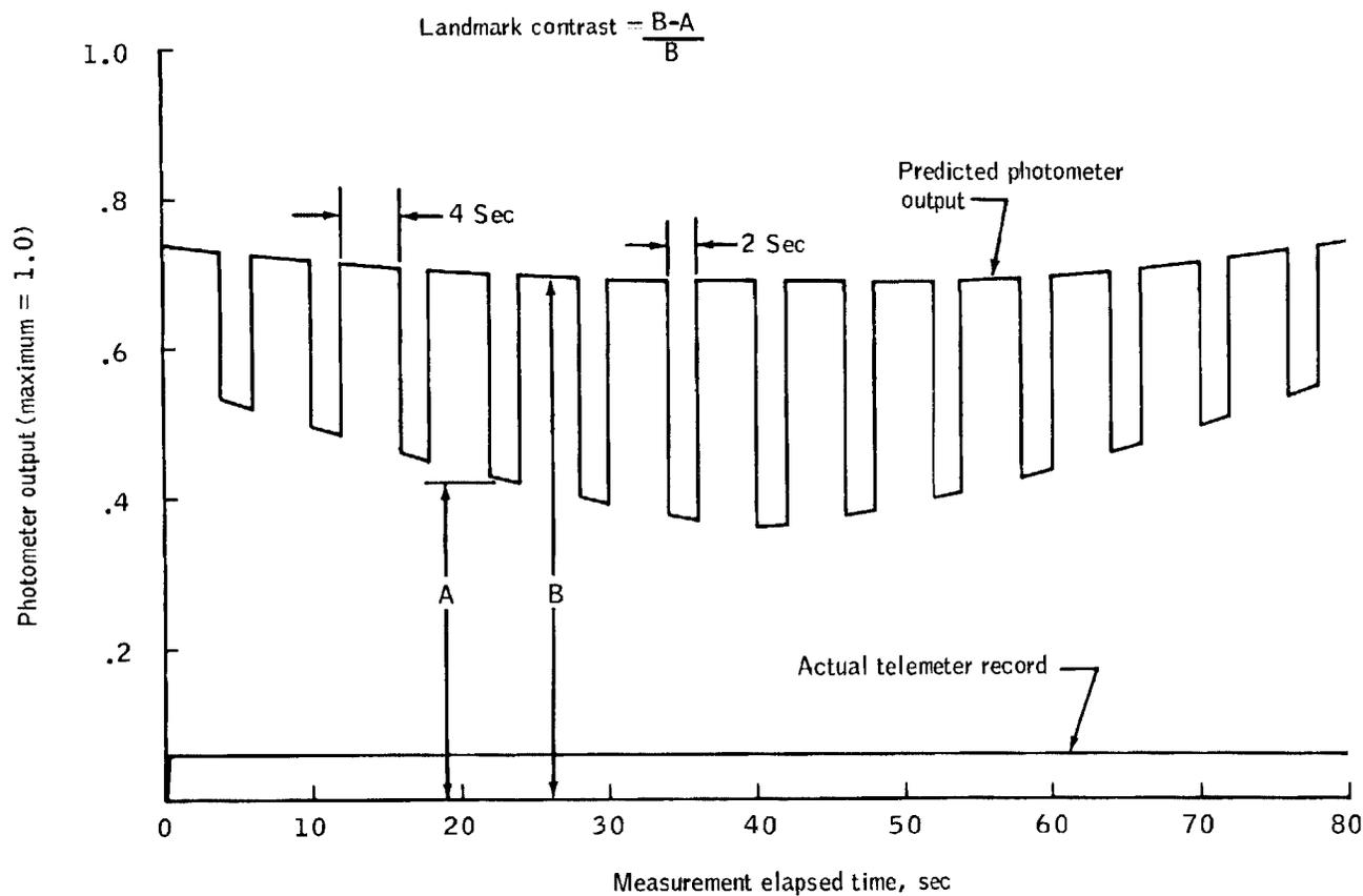
Figure 8.15-2. - Experiment MSC-12 - typical predicted photometer output compared to actual telemeter record.
