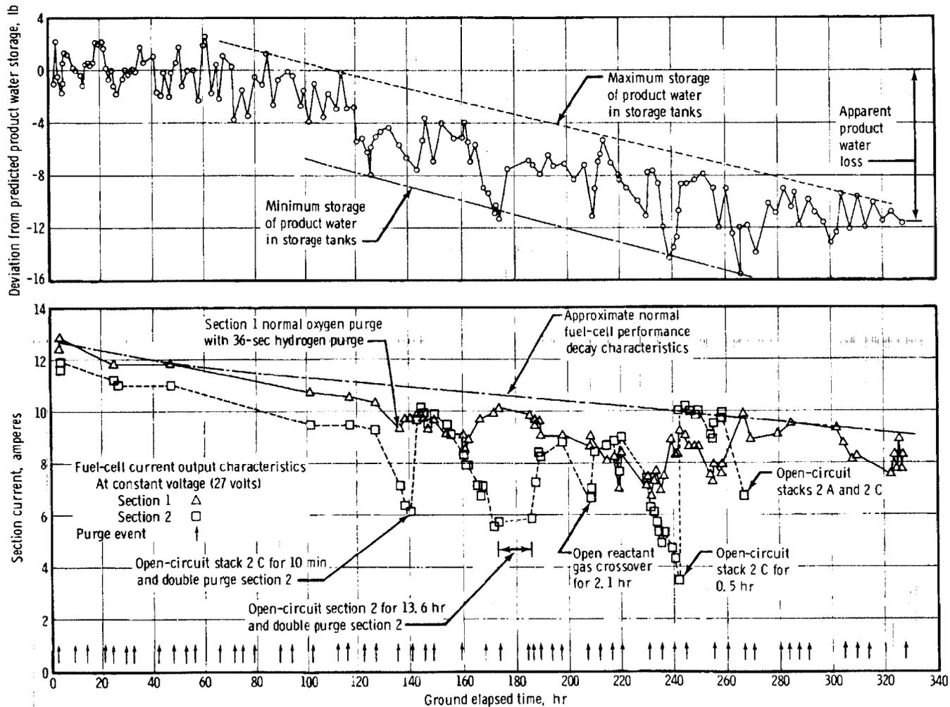
Figure 5.1. 7-4. - Comparison of fuel cell performance with fuel cell product water storage.
