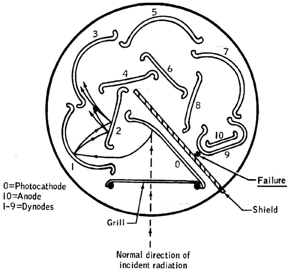
Figure 8.2-1. - Experiment D-5, sketch showing location of photomultiplier tube failure.
