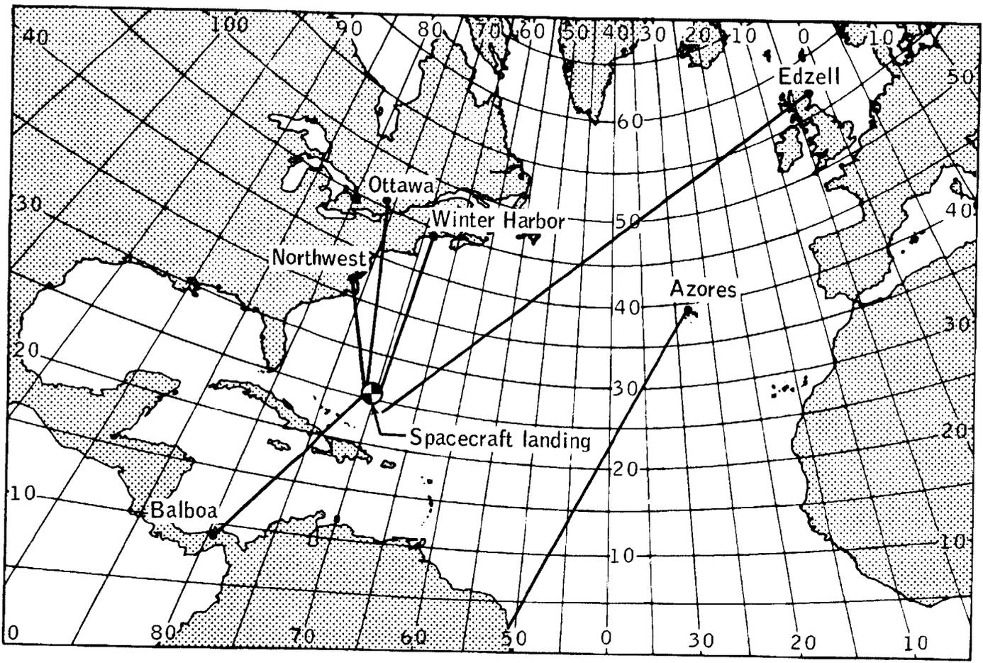
Figure 6.3-7. - HF-DF network station bearings to the spacecraft after landing.
