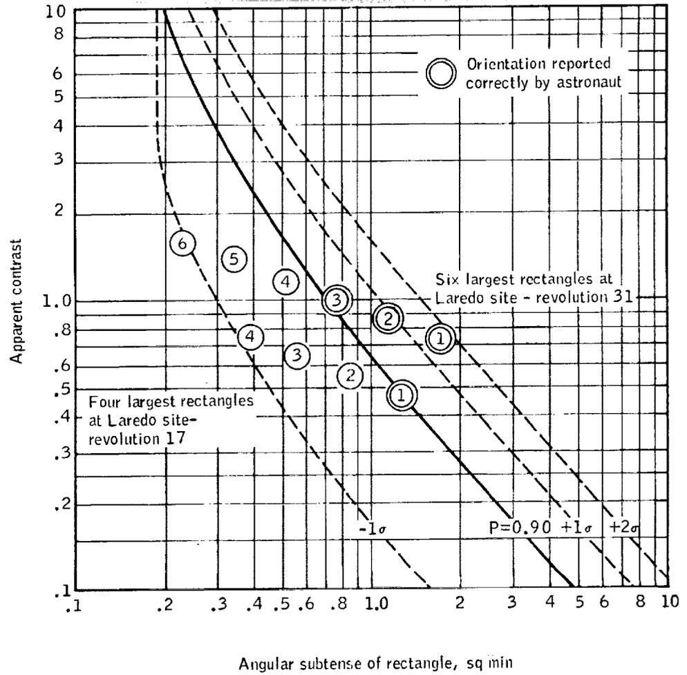
Figure 8.18-2. - Experiment S-8/D-13, preflight visual thresholds, command pilot.
