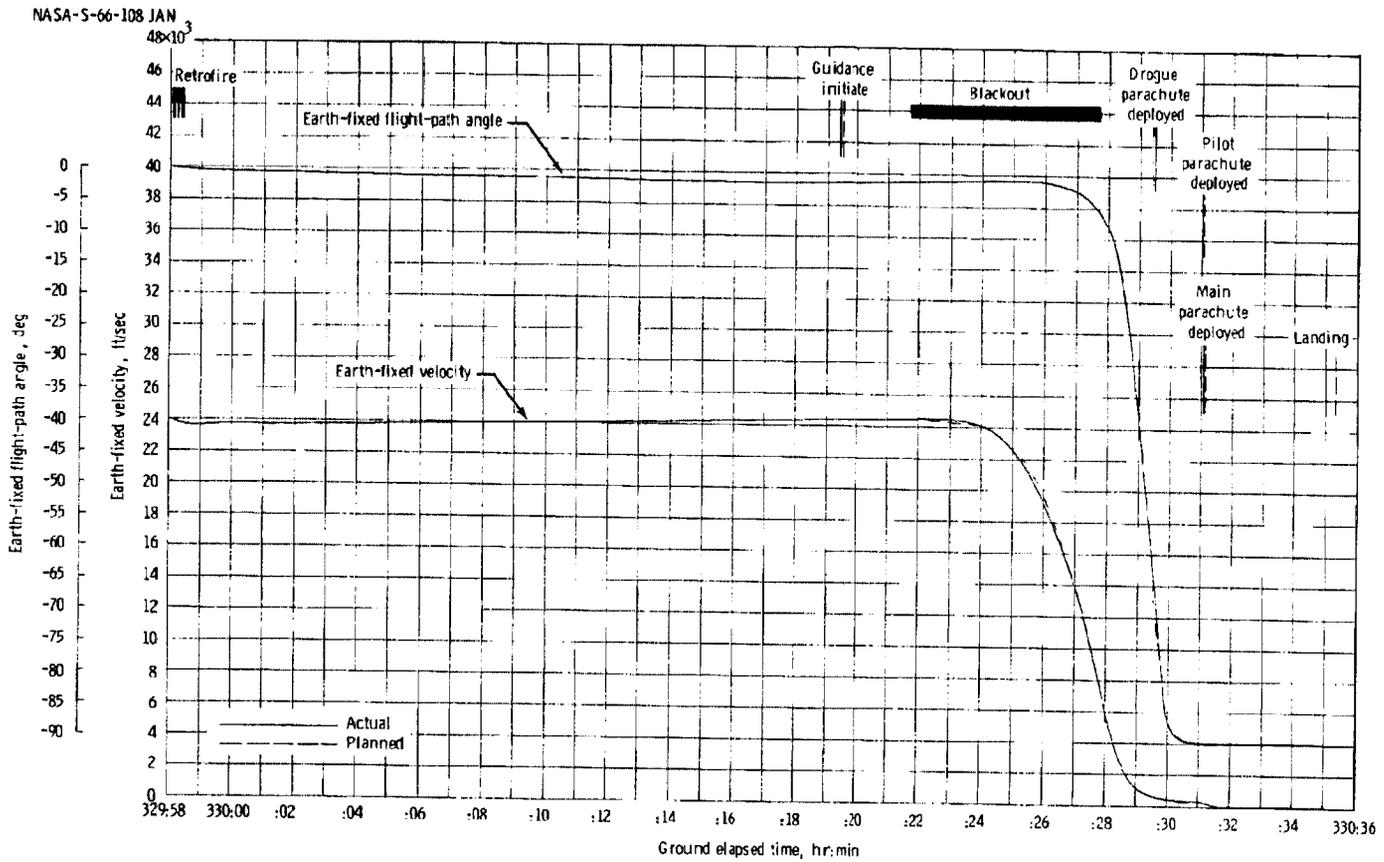
(c) Earth-fixed velocity and flight-path angle.
