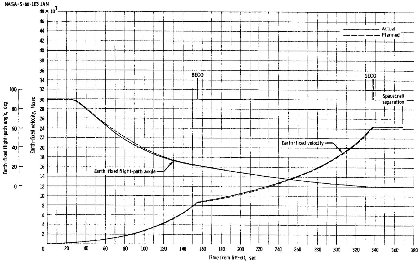
(c) Earth-fixed velocity and flight-path angle.
