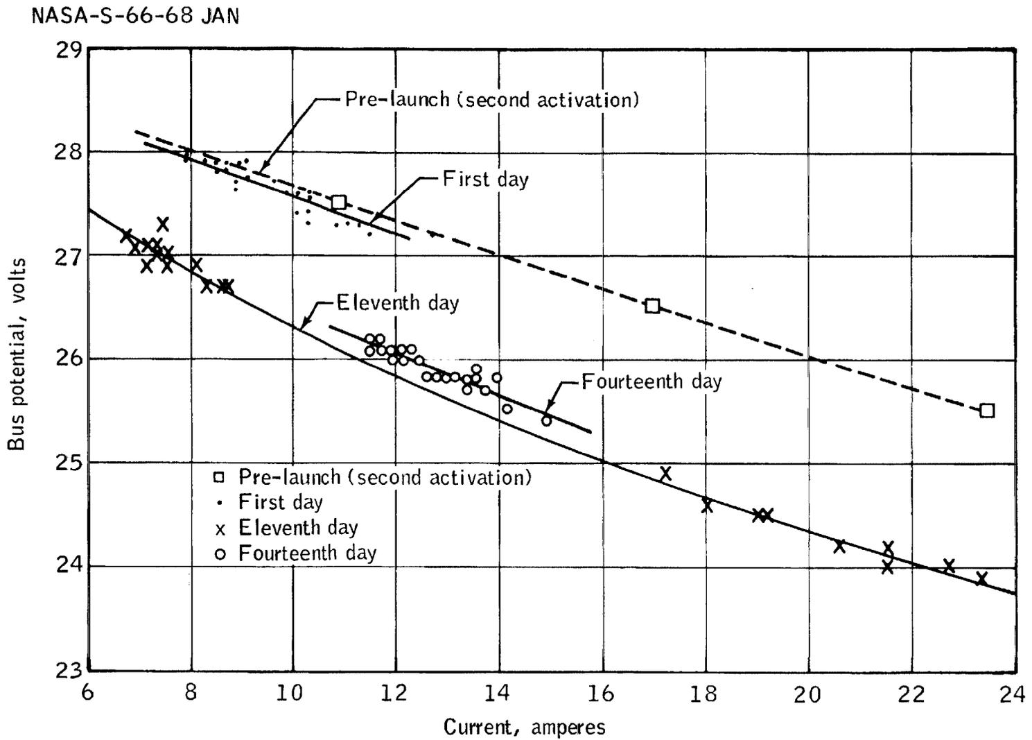
Figure 5.1.7-1. - Fuel cell section 1 performance.
