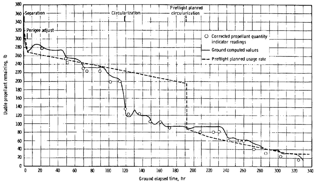
Figure 5.1.8-1 - OAMS propellant consumption.
