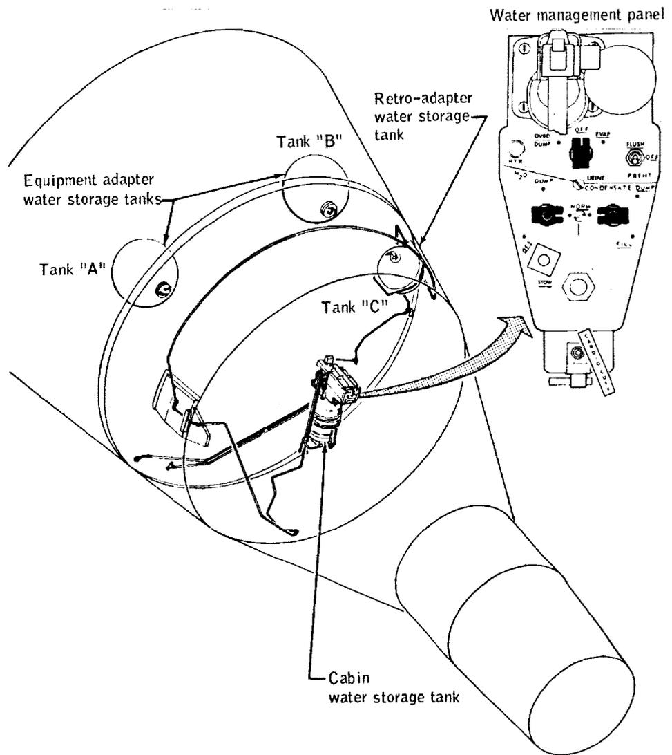
Figure 3.1-4. - Water management system components.
