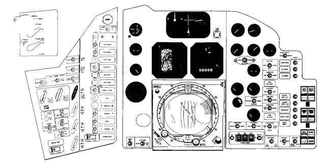
FIGURE 2-3. Main instrument panel and consoles for MR-4 spacecraft.
