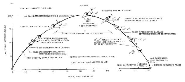
FIGURE 2-5. Flight profile for MR-4.
