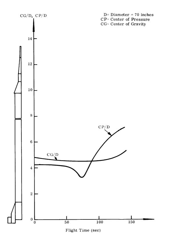
Figure 4-11. MERCURY-REDSTONE Center of Gravity and Center of Pressure Location During Time of Flight
