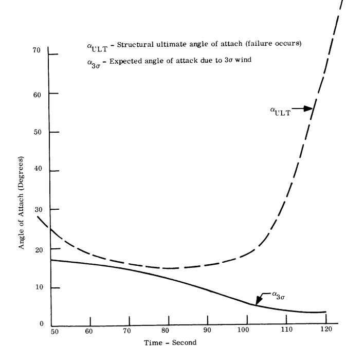
Figure 4-17. MERCURY-REDSTONE Comparison of Angle of Attack versus Time
