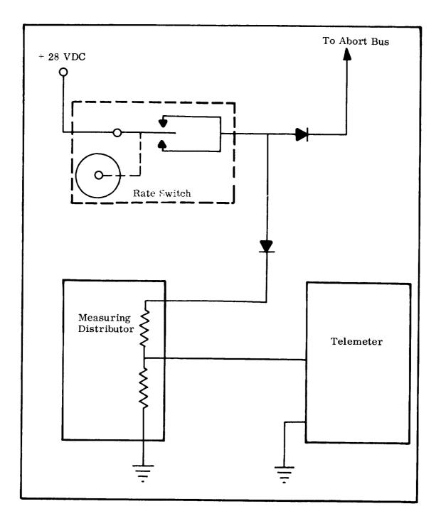
Figure 5-12. Attitude Rate Switch Block Diagram
