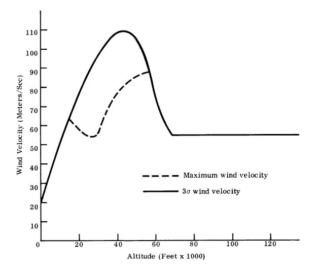
Figure 4-14. Maximum Design Wind Velocity versus Altitude
