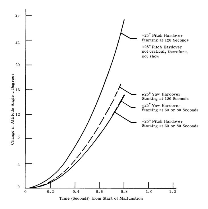
Figure 4-19. MERCURY-REDSTONE Effects of Yaw and Pitch Hardover on Vehicle Attitude Angle (As a Function of Flight Time)
