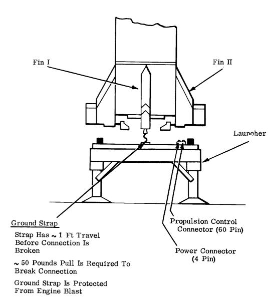
Figure 4-25. Ground Strap Function Just After Liftoff
