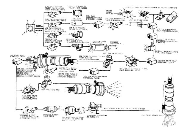
Figure 4-4. Engine Starting Sequence Diagram
