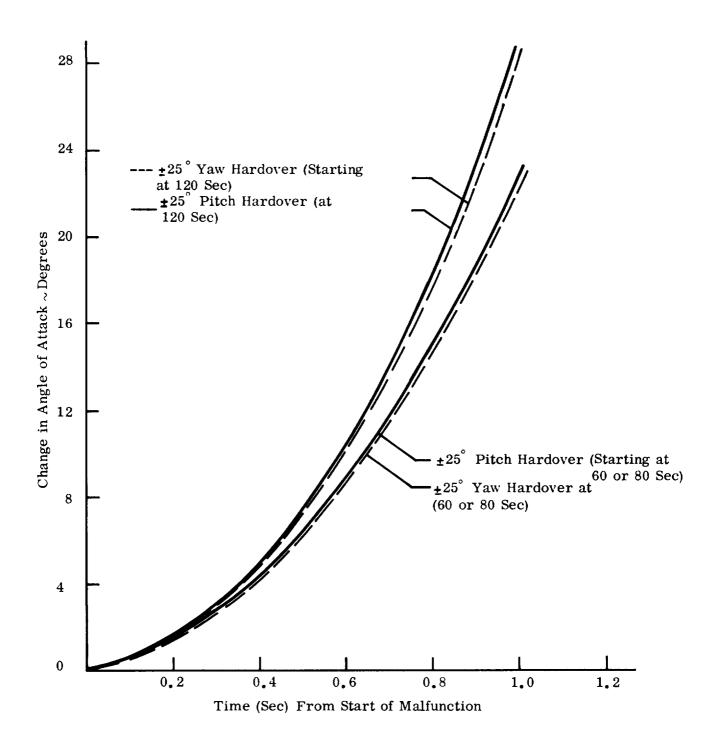
Figure 4-18. Effects of Pitch and Yaw Hardover on Vehicle Angle of Attack (As a Function of Flight Time)
