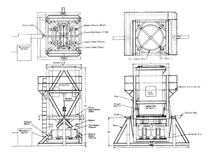
Figure 6-3. Vertical Test Fixtures
