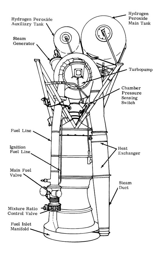
Figure 4-3. A-7 Rocket Engine
