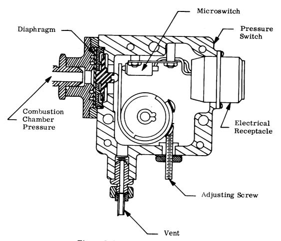
Figure 5-15. Chamber Pressure Sensor
