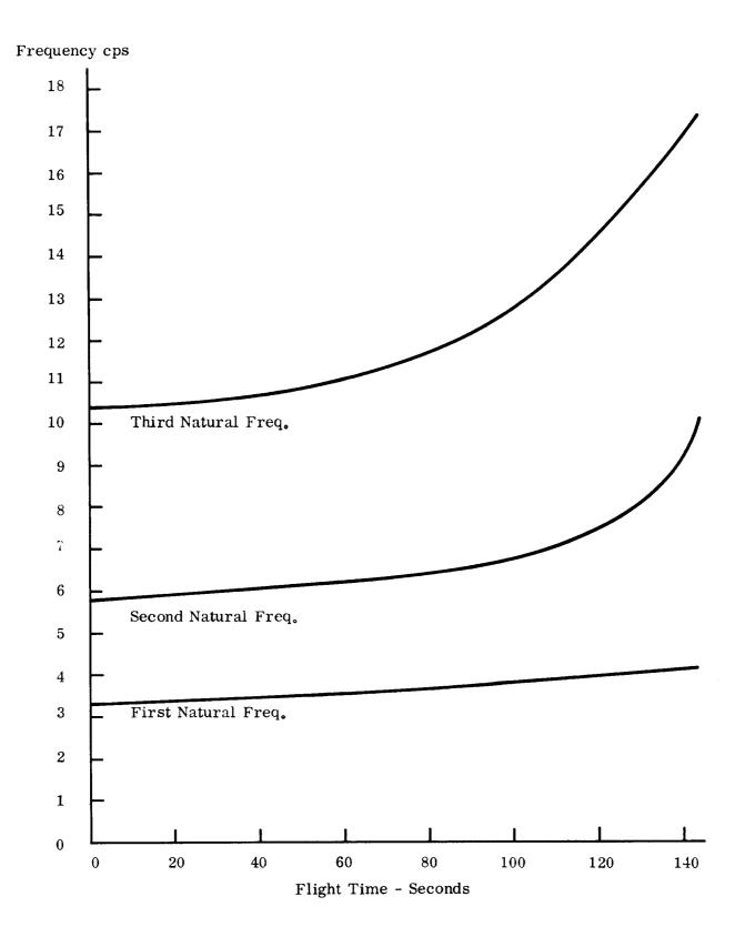
Figure 4-15. MERCURY-REDSTONE Free-Free Lateral Bending Natural Frequency versus Flight Time
