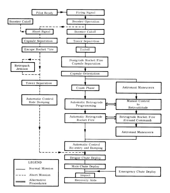
Figure 3-5. Block Diagram of MERCURY-REDSTONE Mission Sequence
