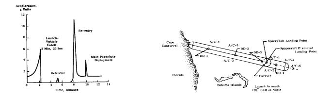
Figure 8-11. Acceleration Time History Figure 8-12. Chart of Recovery for MR-4 Flight
