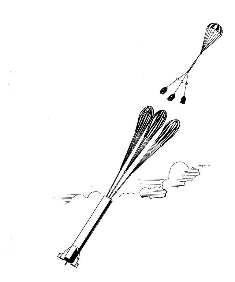
Figure 6-11. Release of Deceleration Parachute and Deployment of Final Recovery Parachutes
