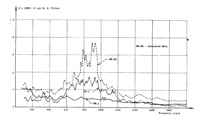
Figure 6-8. Longitudinal Vibration Spectra for MERCURY-REDSTONE Vehicles
