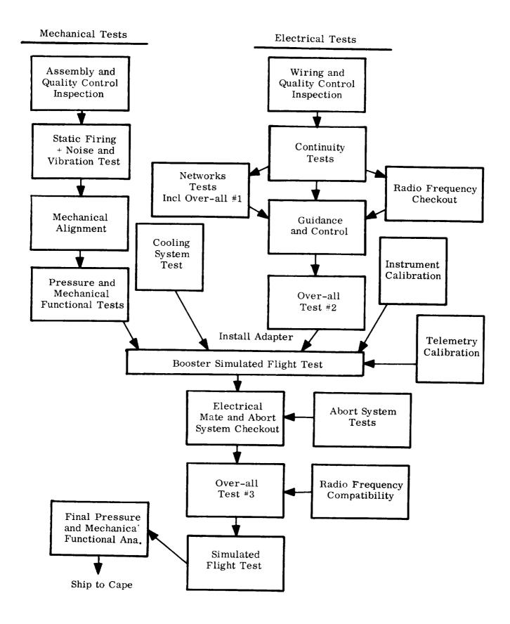
Figure 6-1. MERCURY-REDSTONE System Test Flow Diagram
