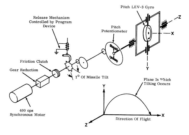
Figure 4-8. Mechanics of Tilting Program
