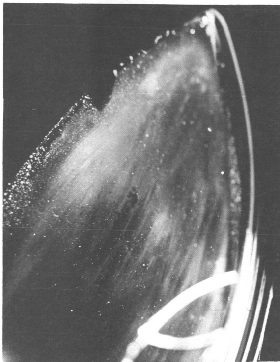
Figure 16. - The Gemini window taken at a sun angle that accentuates the window deposits.
