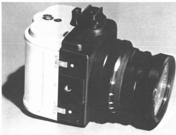
Figure 5. - Hasselblad 70-millimeter super-wide-angle camera with 38-millimeter lens.
