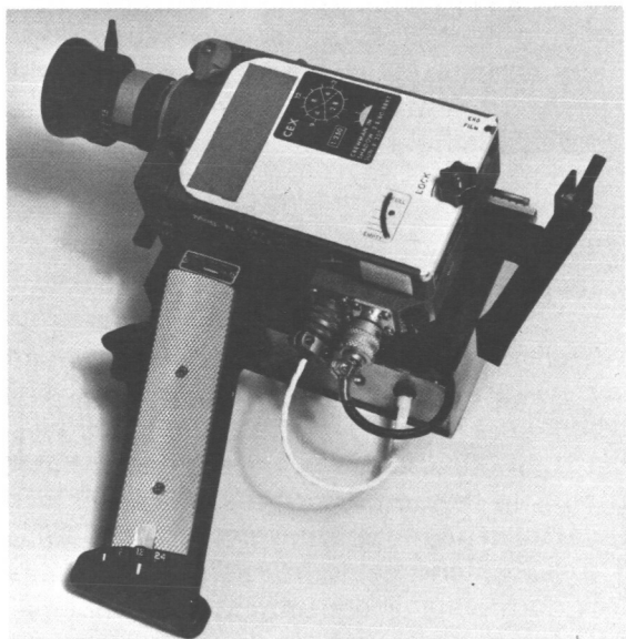
Figure 53. - The 16-millimeter lunar surface DAC system consisting of camera, 10-millimeter lens, camera handle, battery pack, and mounting bracket.
