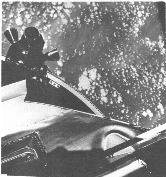
Figure 33. - Lunar module docked with command module, showing condition of LM thrusters and skin.
