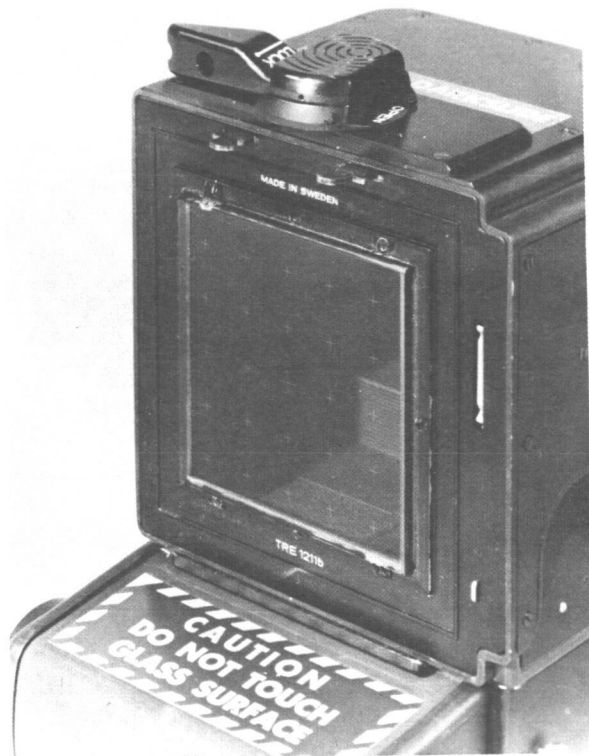
Figure 20. - Reseau plate on 70-millimeter data camera.
